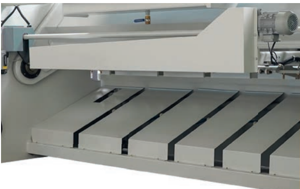
Pneumatic Sheet Support System (Rear Type), (optional)
