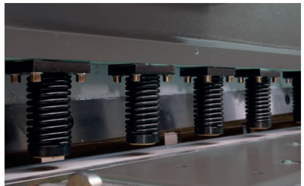
Hydraulic Hold-Down Pads
