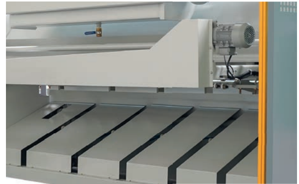
Rear Light Barrier (Standard) Rear Light Curtain (Optional)
